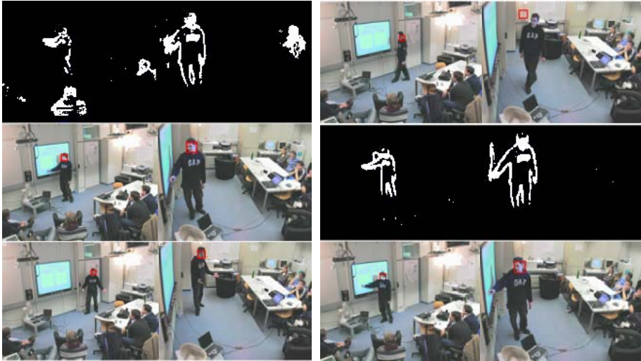
Fig. 5. Typical operation of the proposed multicamera face detection and tracking system. Depicted in left column: Frame 1: Motion analysis. Frame 5: Tracking initialization. Frame 283: Continued tracking. Right column: Frame 324: Lost tracking detected. Frame 331: Foreground segmented by motion analysis. Frame 334: Tracking re-initialization
