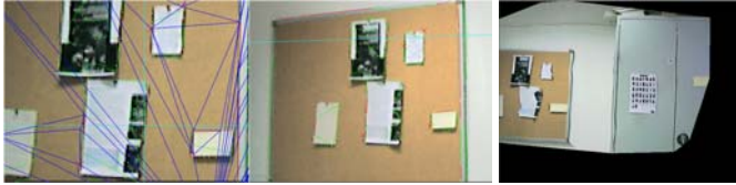
Fig. 2. Left: The Delaunay triangulation for the currently selected point pairs. Quickly zooming in allows for faster and more accurate operation. Middle: Corners and edges visualized on the reference backgrounds. Right: Partially completed rough 3D model, seen from an extrapolated viewpoint at the left side of the inputs
