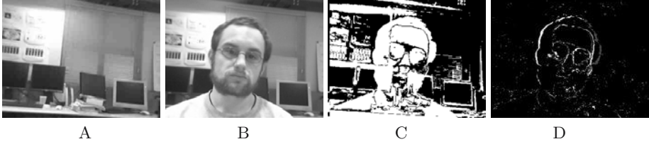
Fig. 1. Images used by our system. A) Background image. B) Example input frame. C) Foreground image I_{f,t} computed from differencing images in A and B (here noisy due to camera shift). D) The signed difference I_{f,t} - I_{f,t-1} . The gray pixels represent I_{b \rightarrow f} , the white pixels represent I_{f \rightarrow b}
