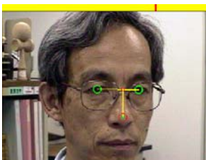
Fig. 3. Example of facial orientation estimation
