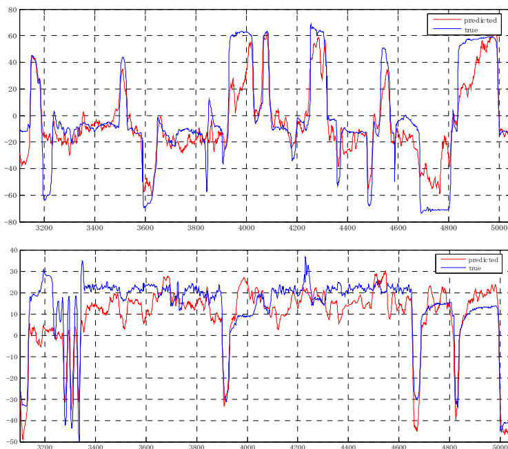
Fig. 6. Trajectories of true (red) and predicted (blue) views obtained by IsoScale for the facial gesture test sequence shown in Fig. 5, with pan (top) and tilt (bottom) measured in degrees
