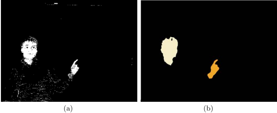
Fig. 2. (a) Result of skin color analysis without post-processing. (b) Result of skin color analysis after post-processing
