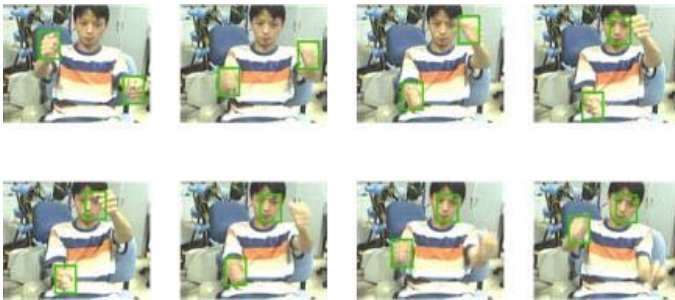
Fig. 4. Tracking failure by color and motion based Mean Shift algorithm
