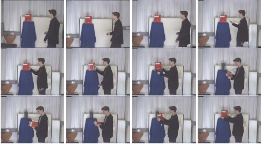
Fig. 6. The first two images are the inputs for the first frame. The other images show several frames of an interpolation result. The virtual camera is located in the middle of the baseline between the two input cameras
